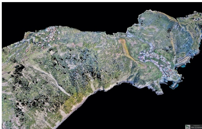
Figure 3. 3D model obtained through the combined use of different survey techniques such as GNSS, Terrestrial Laser Scanner and UAV Photogrammetry
